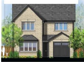
Maidstone - Detached 4 bedroom unit with projecting gable, bay window and integral garage
